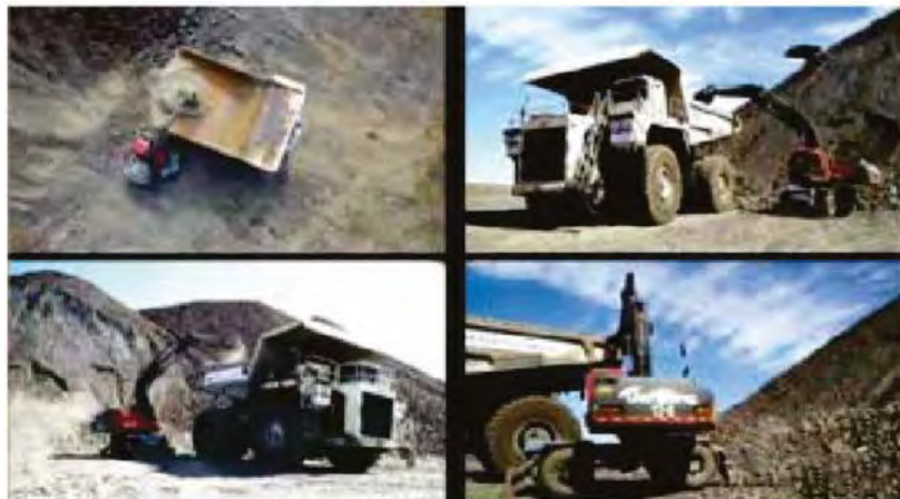
Figure 2-17: 5G-based unmanned mining vehicle operations
