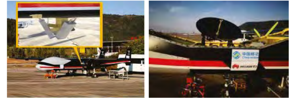
Figure 11-12: World's first flight of an emergency communications sky base station
