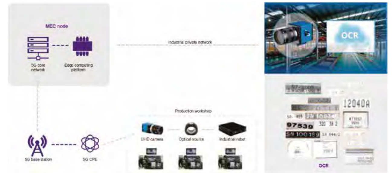
Figure 1-7: OCR applications based on 5G networks
