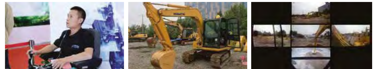
Figure 1-18: Remote excavator powered by 5G
