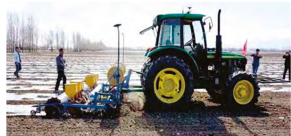
Figure 9-13: Automatic film laying by machinery at a corps in Xinjiang
