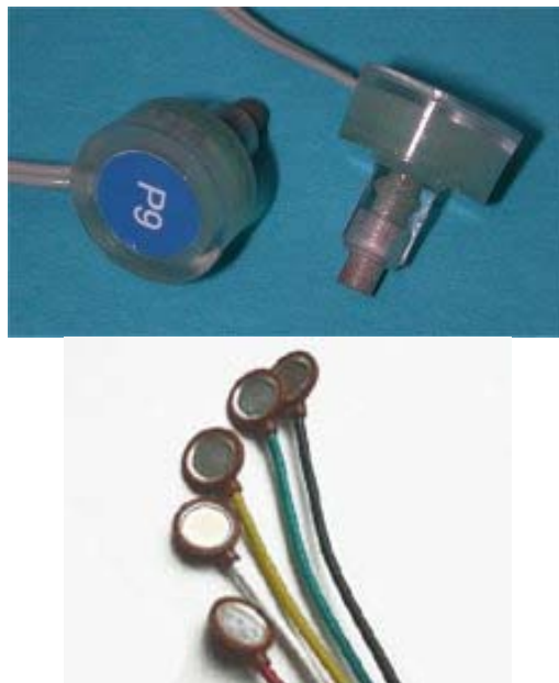
Figure 4.7: Active electrode from Biosemi™ (left), and Ag/AgCl electrode from Nihon Khoden (right). (Source: WWW).
