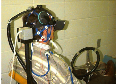
Figure 4.15 : The Rochester BMI. The subject is immersed in a driving environment controlling the car. (Reproduced from Bayliss & Ballard, 2000).
