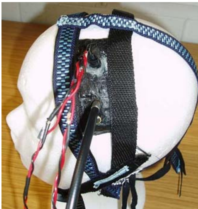
Figure 7.10: Home-made source-detector pair mounted with straps on a mockup head. (Source: WWW).
