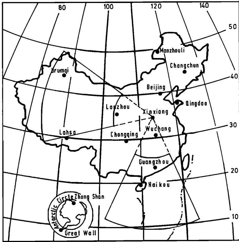
Figure 1. A map showing the coverage of the HF over-the-horizon (OTH) sky wave backscatter radars and the distribution of the Chinese Ionosonde Network (CIN).
