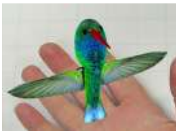
(Left, Above) A Nano Air Vehicle (NAV) (Image courtesy of AeroVironment, Inc.)
