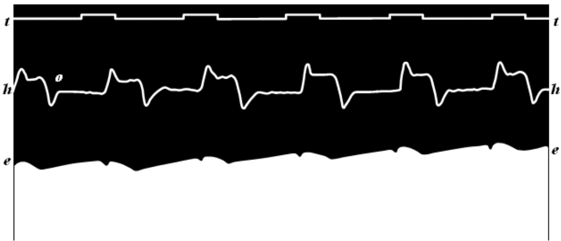
Fig. 1.16. The first recording of the human electrocardiogram by Augustus Waller (1887). The recording was made with a capillary electrometer. The ECG recording (e) is the borderline between the black and white areas. The other curve (h) is the apexcardiogram , a recording of the mechanical movement of the apex of the heart.
